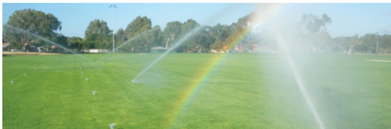
Catch cups can be used to determine precipitation rates and uniformity of irrigation systems
